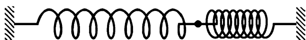
Fig. 3 A widely stretched, weak spring (a polymer) at the left in equilibrium with a slightly stretched, strong spring (a small molecule). Forces at the connecting dot are equal and opposite. The hatched blocks are considered at fixed positions. This represents the interaction of a small-molecule substrate with a binding site anchored on a peptide chain of a protein
